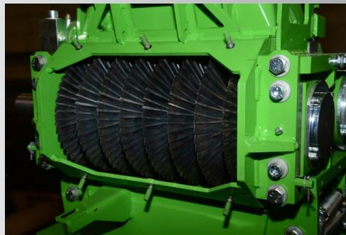
The disc cracker is the guarantee for one hundred percent kernel shredding, even with long chopping lengths without performance-sapping friction floors.
