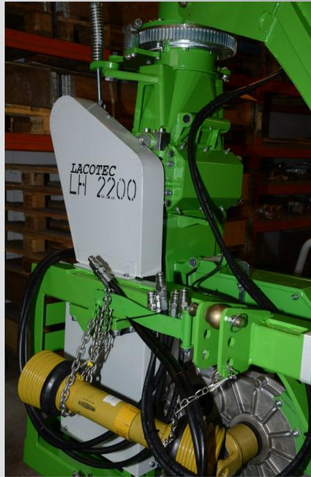
Hydraulic tower controls and chute extensions ensure convenient use with large trailers and a clean forage stream.
