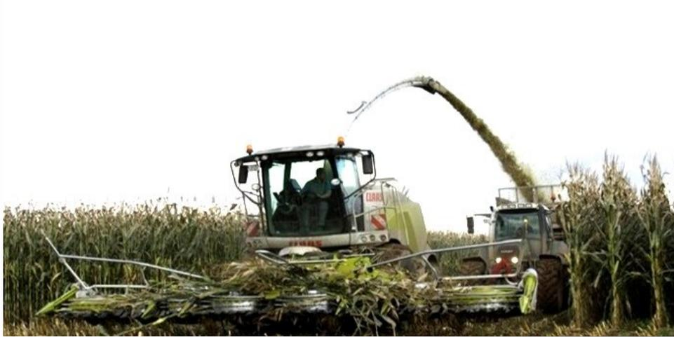
The fact that both rollers run at the same speed, realizes a clean crop flow and accurate delivery of the material to the accelerator, which has a positive effect on throughput and fuel consumption.
