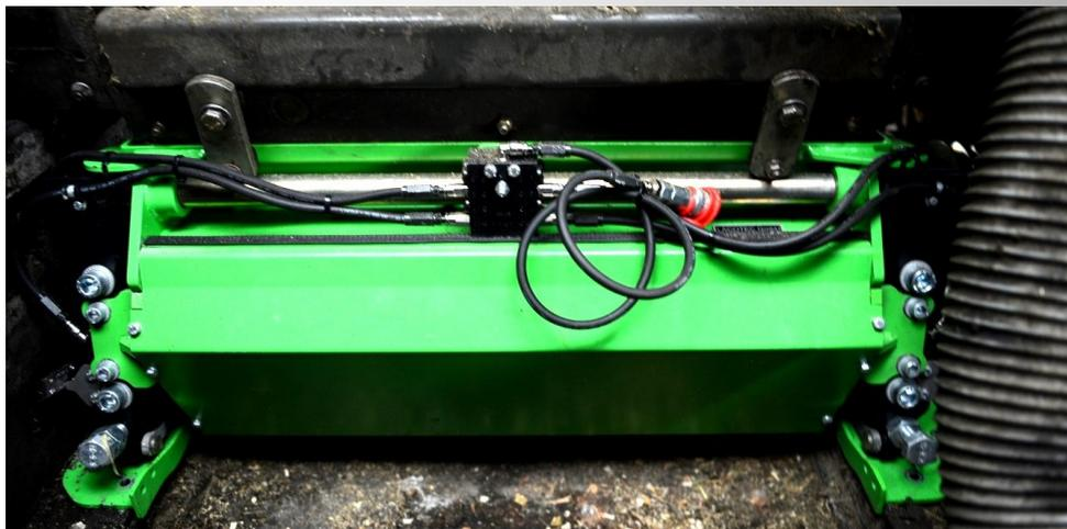
Convenient connection to the central lubrication system.
